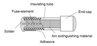
By inserting the fuse-element through openings in the center of SOC's uniquely designed end caps and soldering the fuse-element to the end caps from the outside, we establish firm solder joints and accurately align the fuse-element in the center of the fuse. This construction results in a mechanically robust, highly reliable fuse with low electric characteristic variance.
